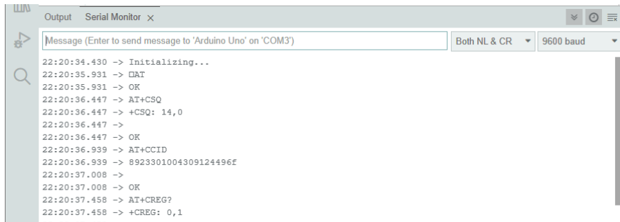
Figure 10: GSM test result captures from Arduino sketch using AT commands
