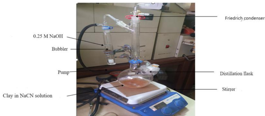
Fig. 2. Device for evaluating cyanide volatility
