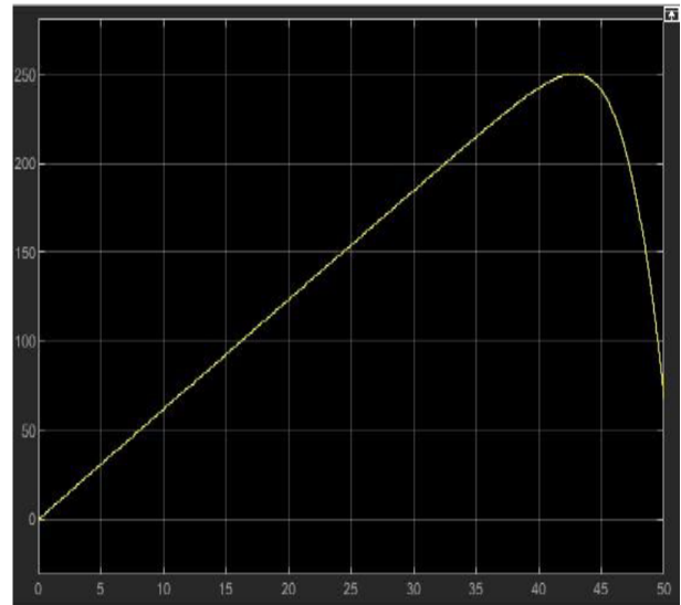
Fig. 2.PV Characteristics of a Solar cell
