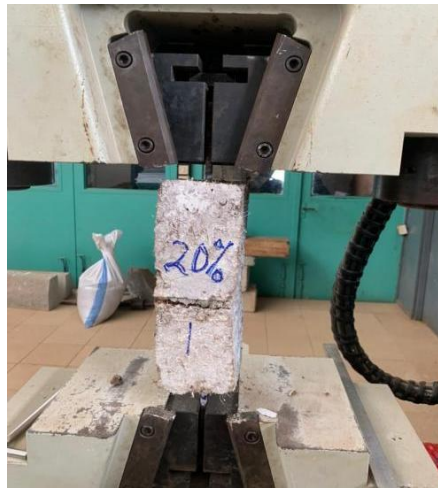
Fig-7: Bond failure mechanism
