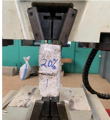
Fig-7: Bond failure mechanism
