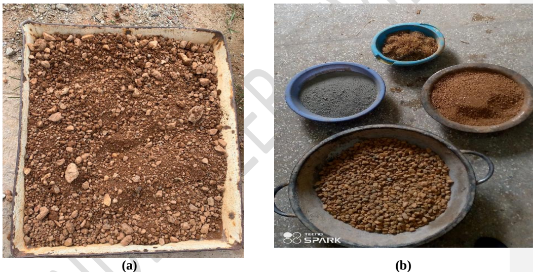
Fig-1: (a) Laterite soil (b) Cement, Fine aggregates, Coarse aggregates and Palm kernel fibre
