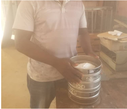
(a) Recycled glass powder on top sieve arranged according to sizes
