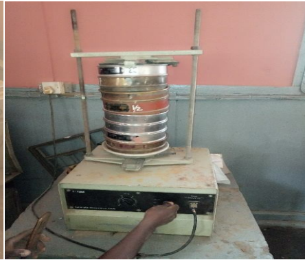
(b) Recycled glass powder and sieves mounted on mechanical shaker
