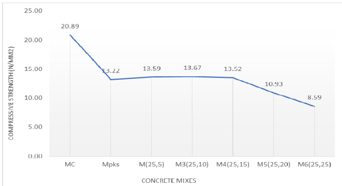
Fig. 20: 7th day compressive concrete strength of various RGP with 25% PKS replacement to granitic coarse aggregate.
