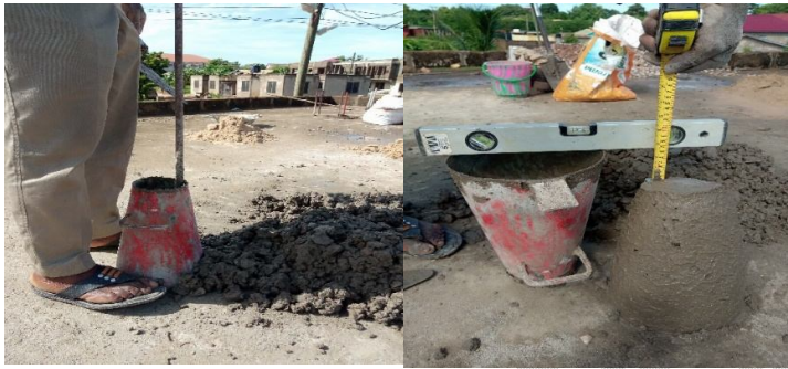
(a)Compacting of concrete sample in slump mold
