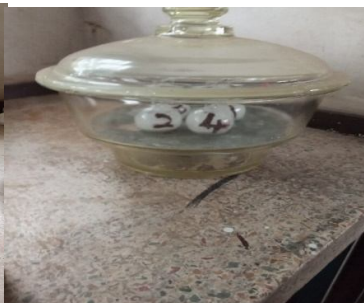
(e) Bottle plus recycled glass powder and water placed in desiccator
