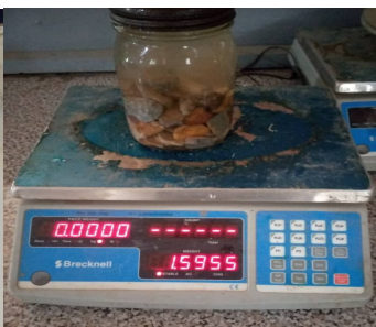
(b) Pyknometer plus water and coarse aggregate weighed
