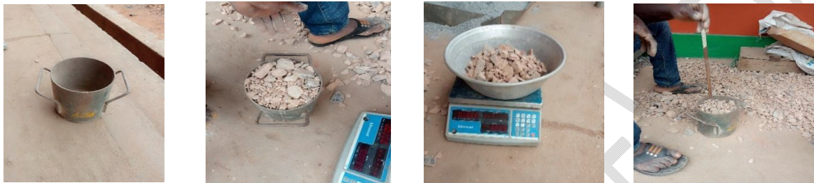
(d) Tamping rod permitted to fall easily from a height of 50mm above the surface of the aggregate
