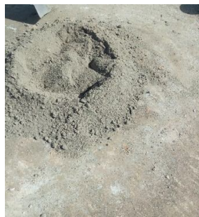
(c) Mixture of cement, recycled glass powder and fine aggregate
