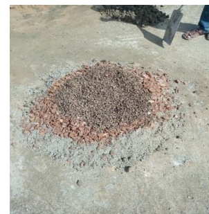
(d) Coarse aggregate and shells of palm kernel added to the mixture of cement, recycled glass powder and fine aggregate
