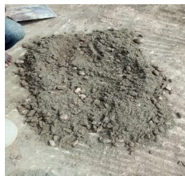
(f) Water added to the mixture of fine aggregate, cement, recycled
