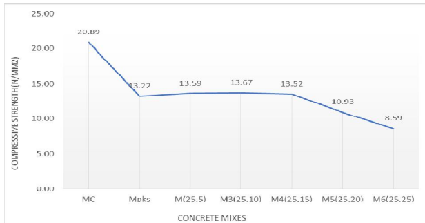
Fig. 20: 7th day compressive concrete strength of various RGP with 25% PKS replacement to granitic coarse aggregate.
